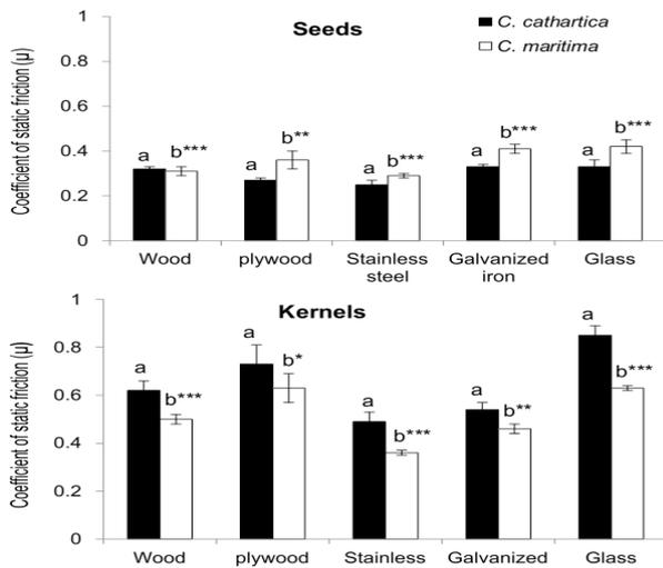
Figure 4. Coefficient of static friction ( $\mu$ ) of seeds and kernels of *Canavalia* (\*,  $p < 0.05$ ; \*\*,  $p < 0.01$ ; \*\*\*,  $p < 0.001$ )
